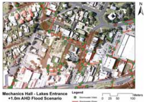
Figure 11. 2D modelled inundation extent image (+1.0 m AHD) for the Mechanics' Hall area, showing contribution of the stormwater network to inner-township floodwater inundation.
