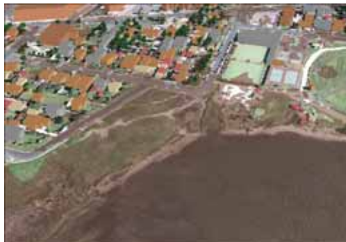
Figure 8. 3D modelled inundation extent image (+1.2 m AHD) for 'The Oval' area of the Lakes Entrance township.
