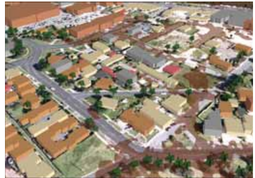
Figure 10. 3D modelled inundation extent image (+1.0 m AHD) for the Mechanics' Hall area of the Lakes Entrance township.
