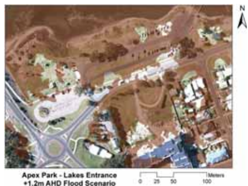
Figure 6. 2D modelled inundation extent image (+1.2 m AHD) for the Apex Park area, Lakes Entrance township.
