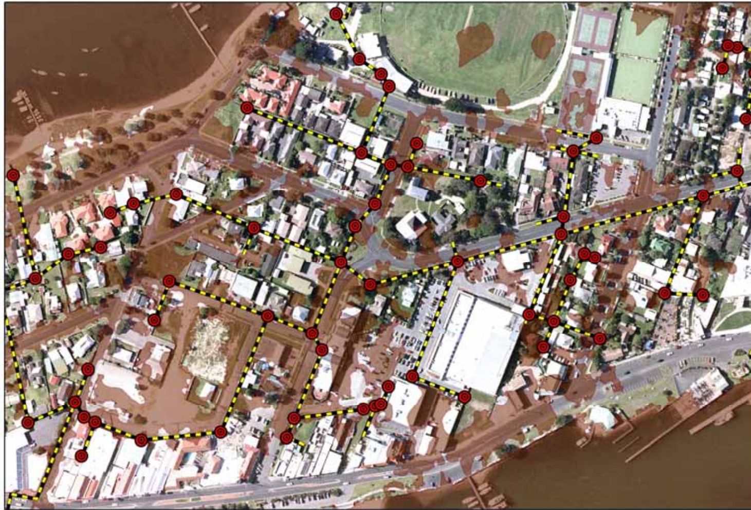
Lakes Entrance +1.2m AHD Flood Scenario 'At-risk' Sewer Assets
